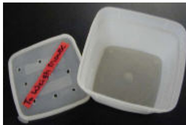
Figure 1. To prevent mice from escaping when weighing them, use a weighing chamber. This one is made from a refrigerator container with air holes punched in the top.
