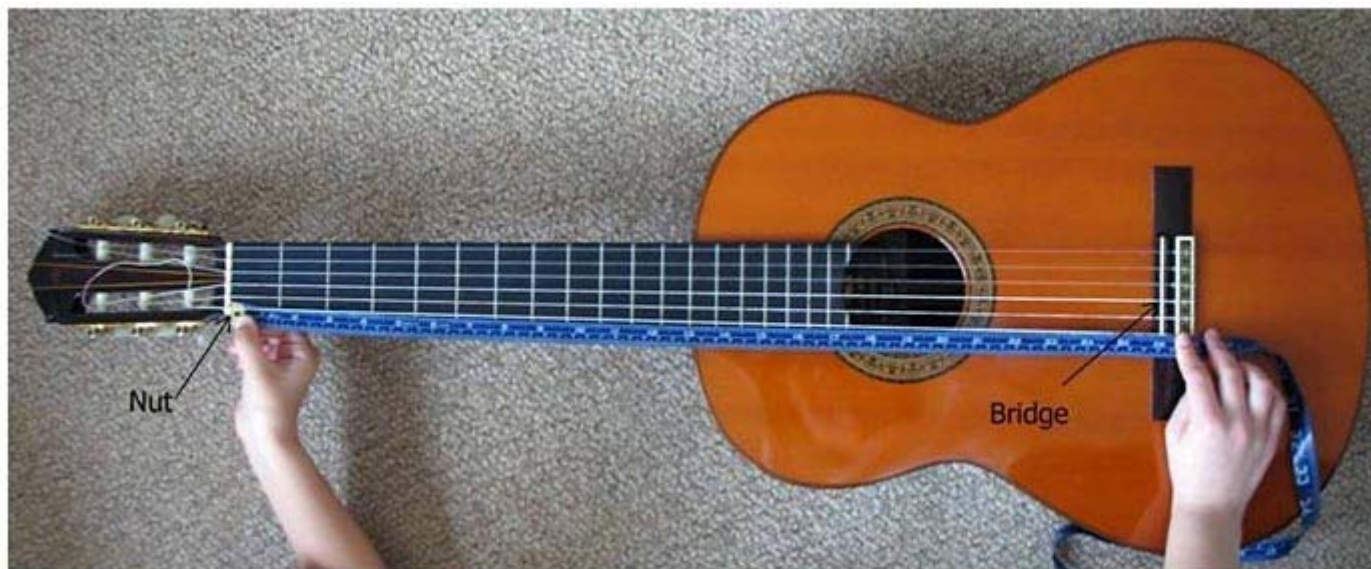
Figure 6. This photo shows how to measure the string length from the nut to the bridge.
