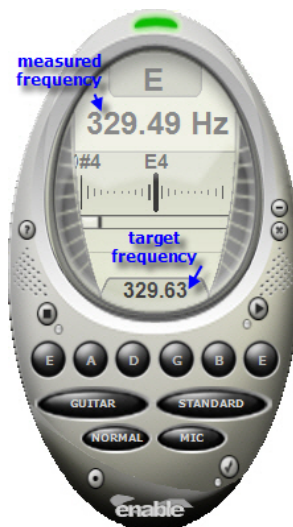
Figure 7. Screenshot of the enable Tuner® software display, showing where to read the measured frequency of the note that was played. The target frequency of the open strings is displayed in the lower portion of the window, as shown.
