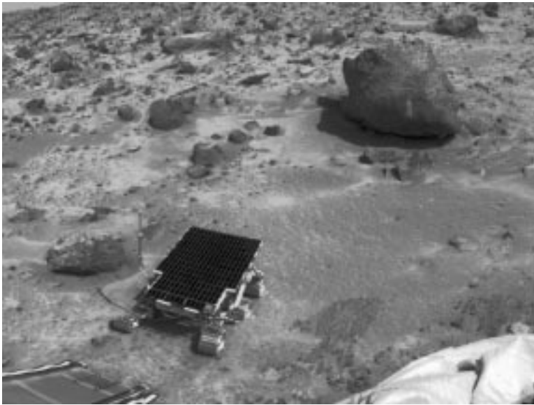
Scale: Rover is 65 cm long, 48 cm wide, and 30 cm tall.
