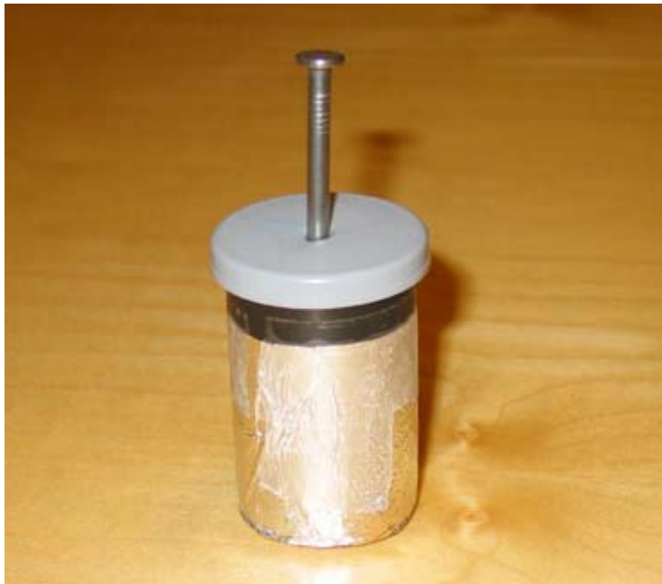
Figure 4. Leyden jar made from a film canister.
